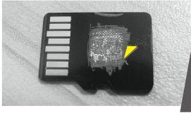
Exposure of Components Caused by Scratching
